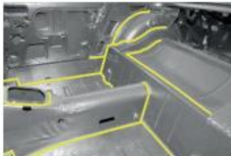
Tunnel and rear body Apply to both sides of the tunnel, down into the footwell, rear floor and rear inner wheel arches.
