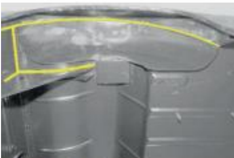
Rear wheel arches Apply to both sides as shown (left hand side illustrated).
